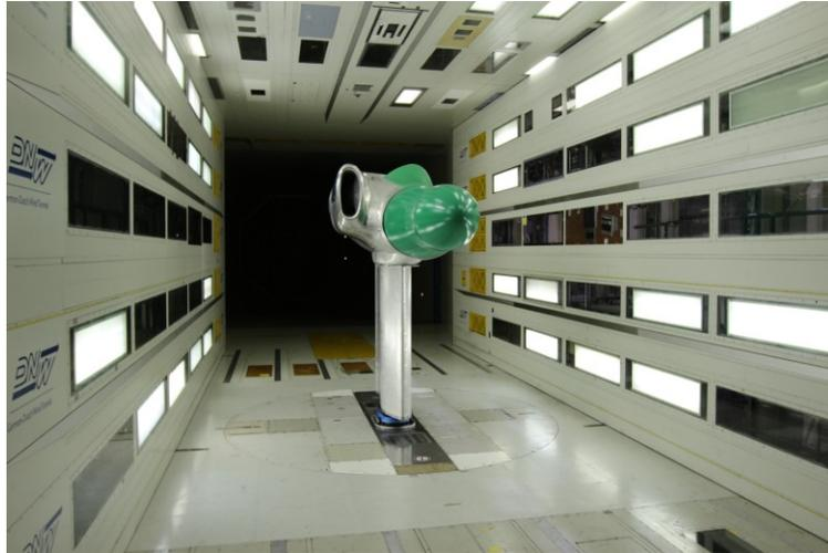
Figure 16 DNW-LLF test section with a full-scale intake geometry.
