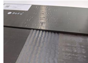
Milled variable thickness weld specimen
