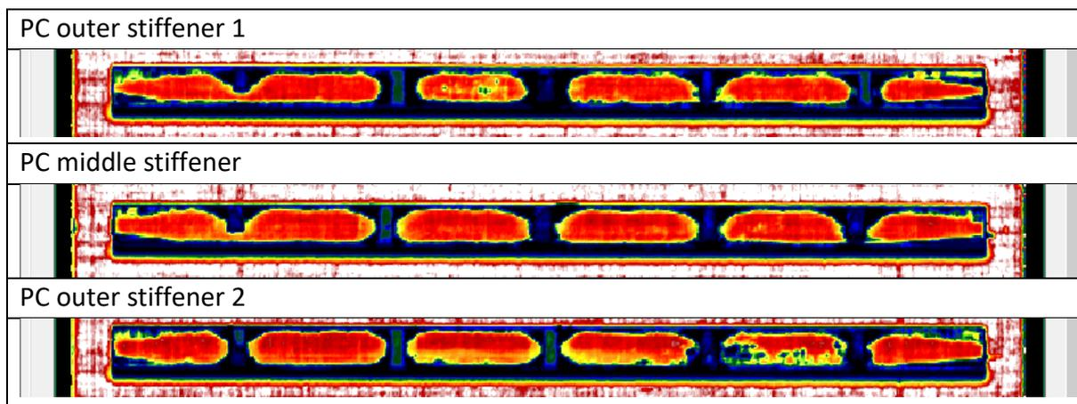
Figure 10: Attenuation scans of welded multiple L-stiffener samples
