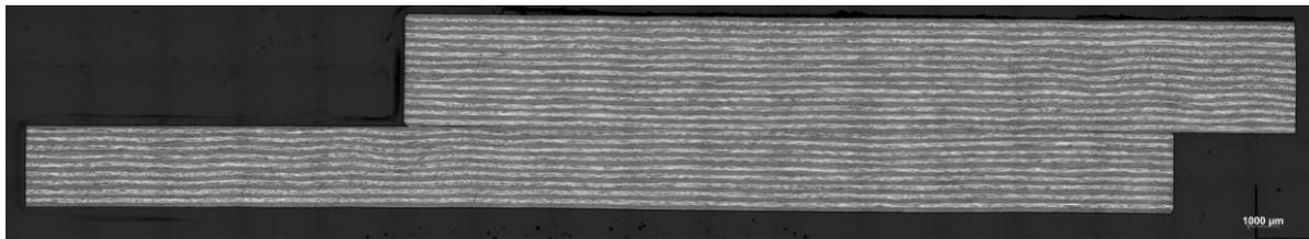
Figure 14: Cross-Section B-B: Weldline width correspond with C-scan (top laminate 3.7 mm, bottom 2.7mm)
