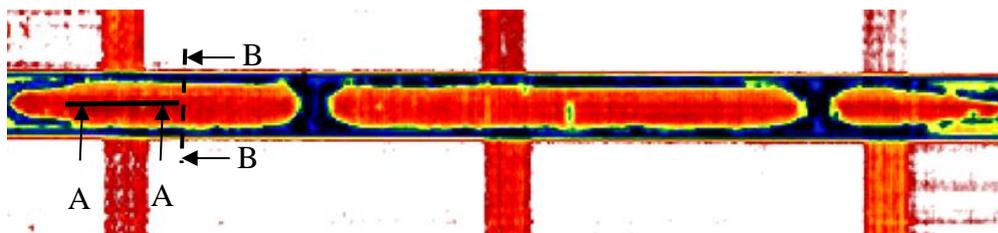
Figure 12: C-scan result of the variable thickness weld specimen
