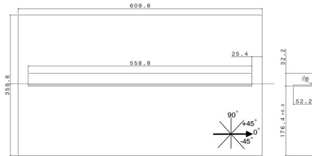
Figure 4: Rosette orientation and dimensions of single L-stiffener samples
