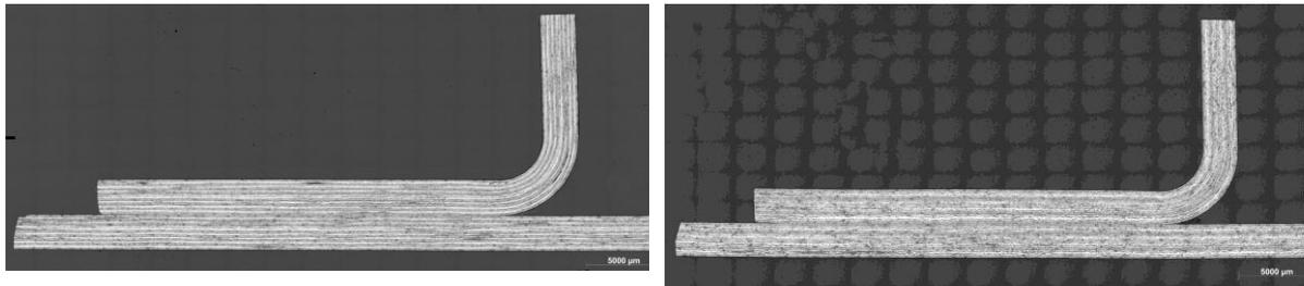
Figure 9: Cross-sections of welded samples (SW set 3 cross-ply left, SW set 4 QI right)
