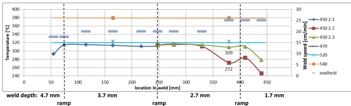
Figure 7: Longitudinal temperature distribution at the weld interface of the 500 mm long variable thickness specimen on each weld depth level at different weld power settings and weld speeds
