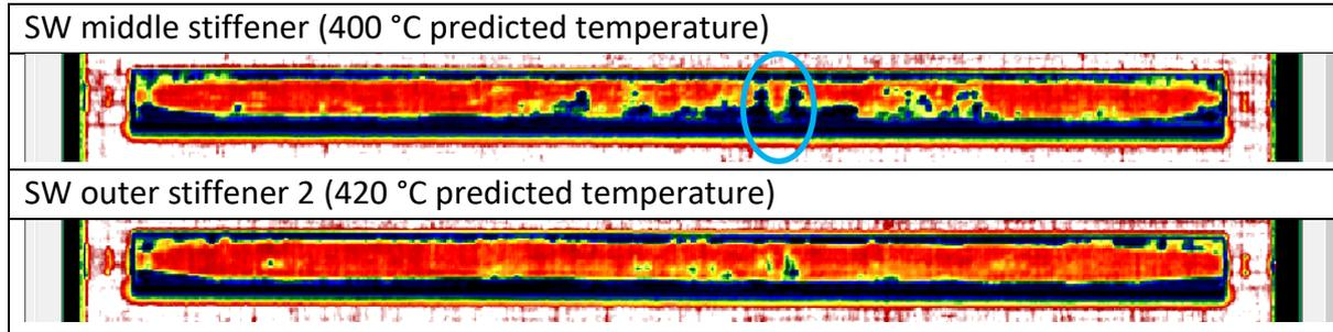
Figure 11: Attenuation scans of welded multiple L-stiffener samples
