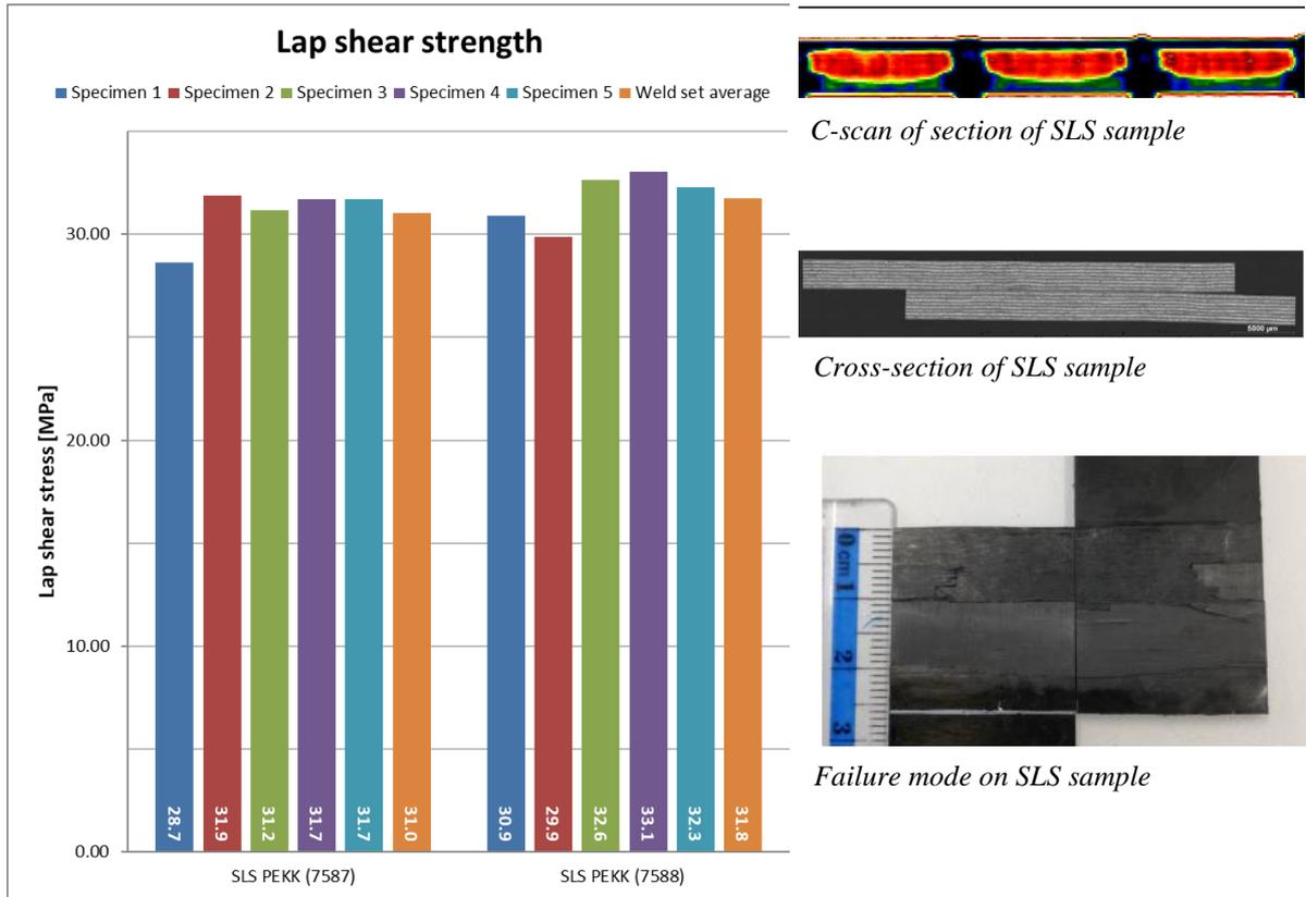
Figure 6: UD PEKK lap shear strength and typical failure mode of SLS specimen
