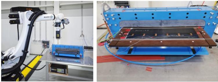
Figure 2: Robotic Induction Welding setup with standard SLS weld tool at NLR
