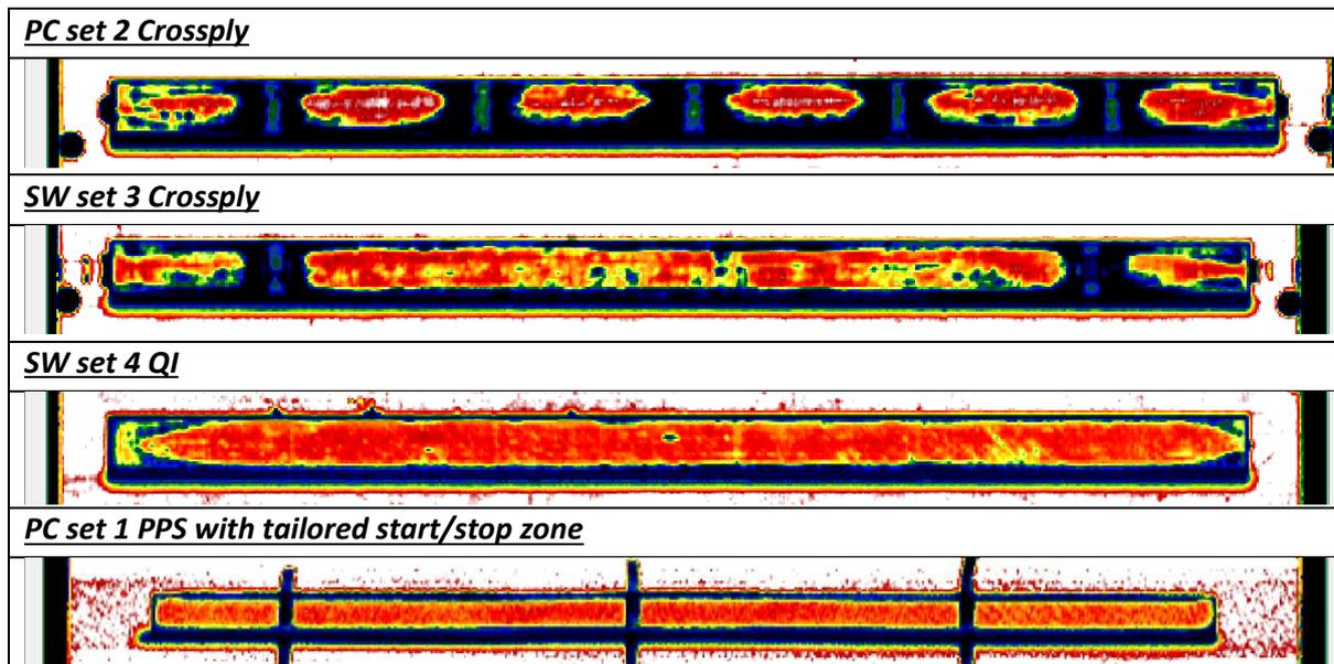
Figure 8: Attenuation scans of welded single L-stiffener samples
