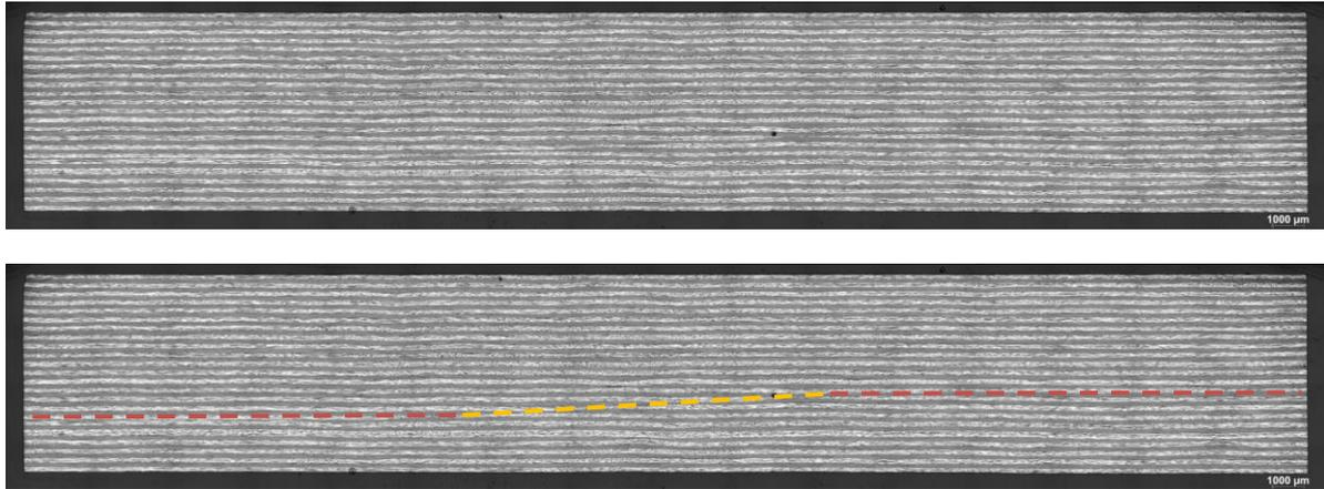
Figure 13: Top; Cross-section A-A: Location of weld interface not visible (top laminate 4.7 mm, bottom 1.7mm, including ramp) Bottom; Same cross-section indicating location of weld interface.
