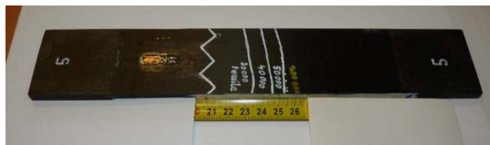
Figure 20: Crack propagation for tension load
